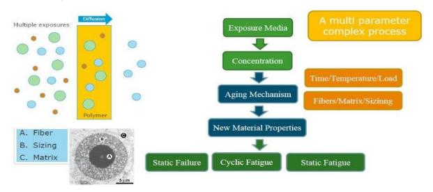
For composite materials such as those used in the reinforcing tape the ageing is more complex due to the different degradation effects on the reinforcing fibres, the matrix and their interface. In order to accurately design a thermoplastic composite pipeline structure that is suitable for operation over a number of years it is imperative that we understand the polymer and composite (tape) performance after it has been degraded through environmental and thermal ageing.
