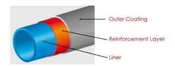
The resulting thermoplastic composite pipeline is flexible and can be spooled and onto a tight radius drum, enabling multi-kilometre lengths of pipe to be stored on a single drum. This spooled pipeline can be deployed at a much faster rate than traditionally welded steel pipelines.
